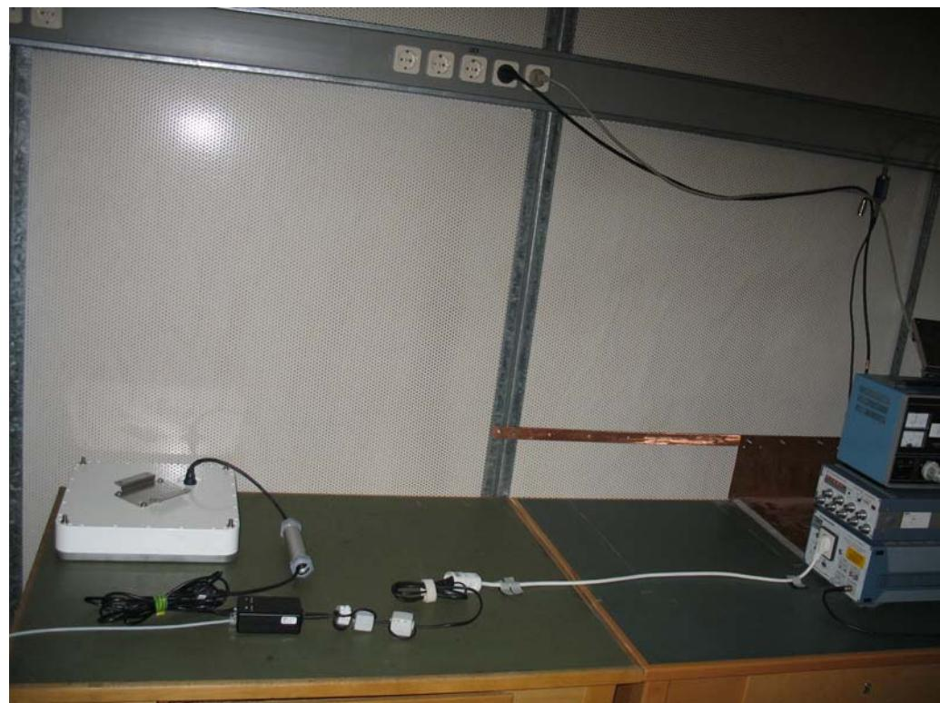
Remark: modification was done by means of using ferrites on the main-lead
