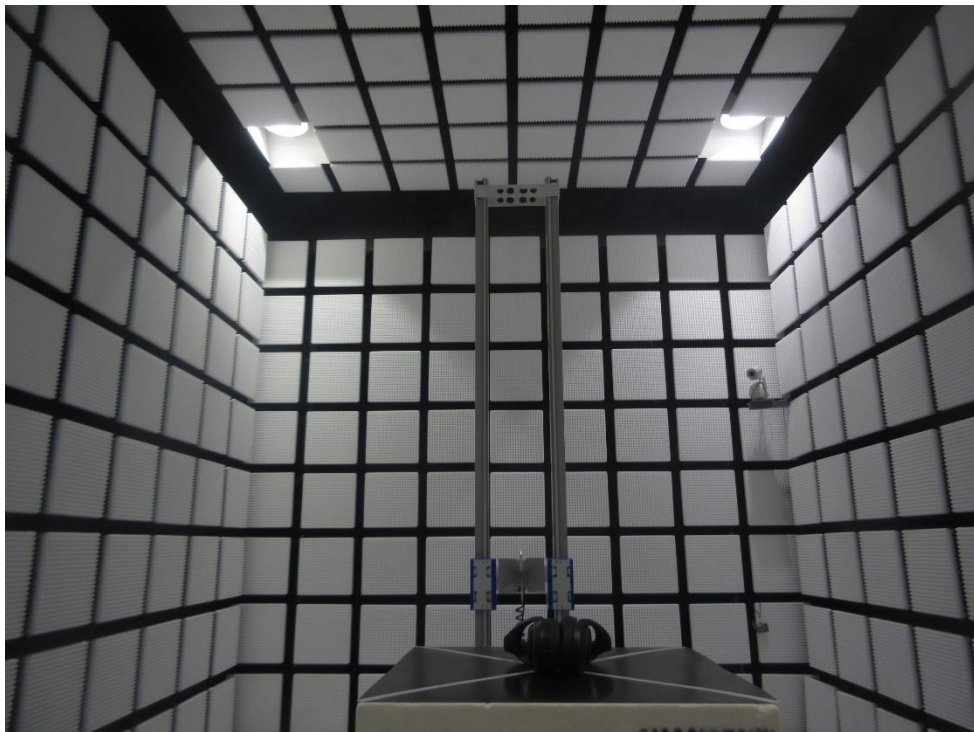
Radiated Spurious Emission Test above 1GHz
