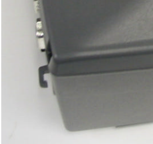
Figure 8 Detail of strain-relief feature
