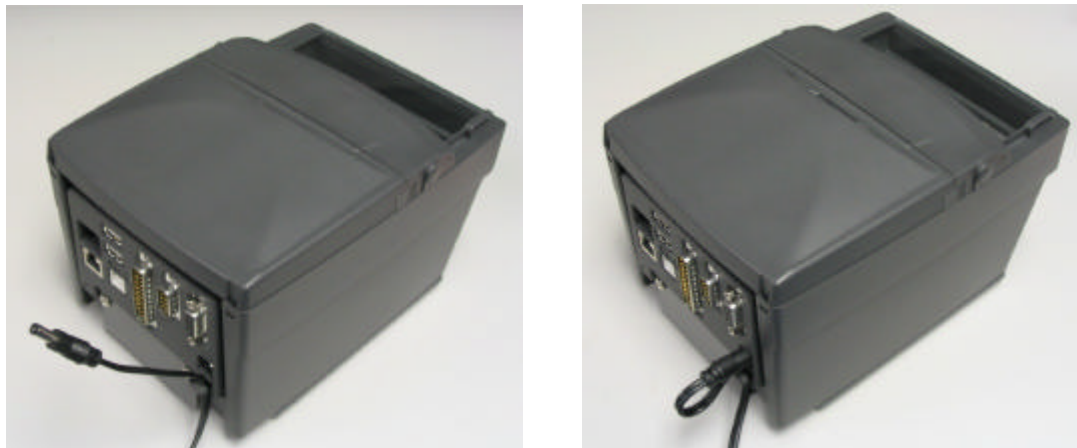
Figure 4 Attaching the power adapter
