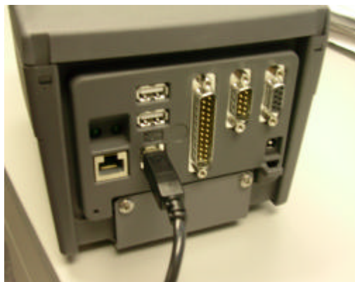
Figure 7 Attaching the USB2.0 cable
