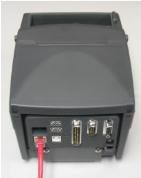
Figure 5 Attaching the ethernet cable
