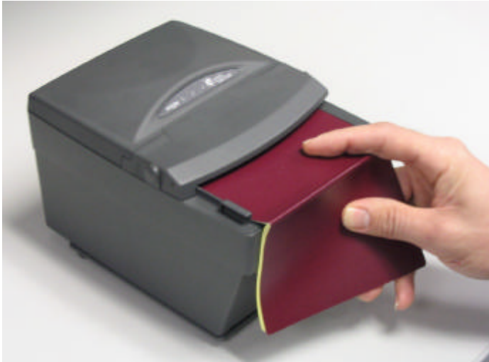
Figure 10 Placement of document on the EAGLE Reader
