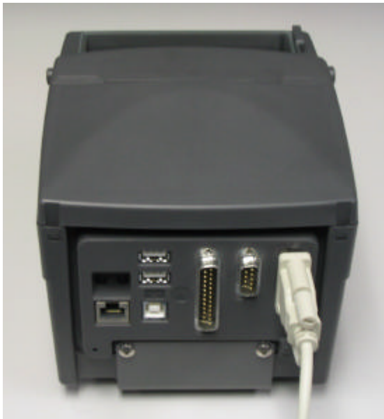
Figure 2 Attaching the serial cable
