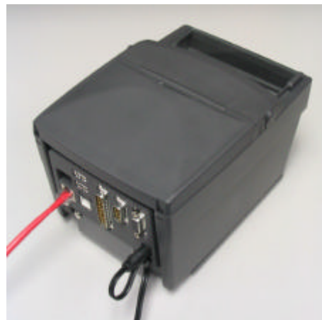
Figure 6 Attaching the power adapter (The power should be connected after all other connections)
