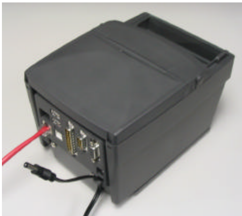
Figure 6 Attaching the power adapter (The power should be connected after all other connections)
