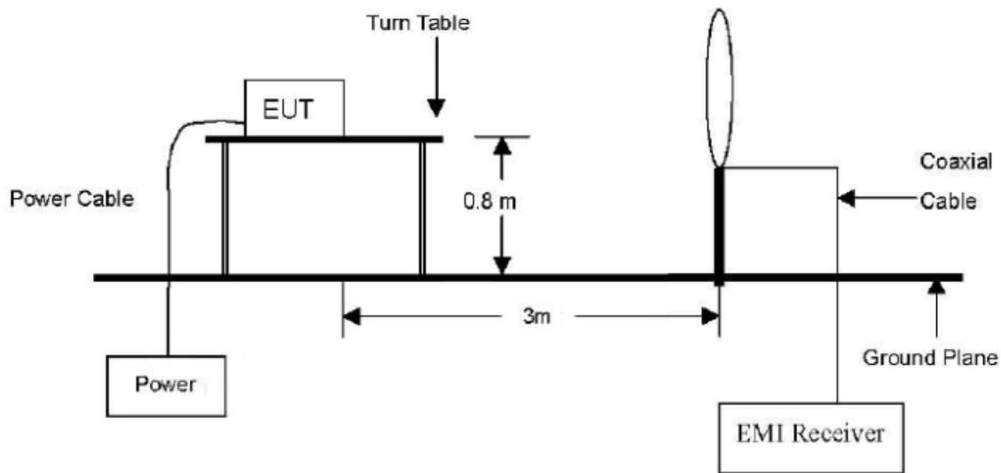
The diagram below shows the test setup that is utilized to make the measurements for emission from 30 MHz to 1 GHz emissions.
