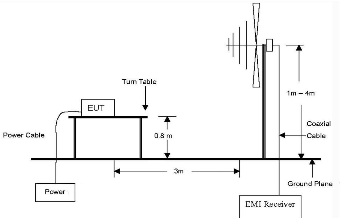
The diagram below shows the test setup that is utilized to make the measurements for emission from 1 GHz to 40 GHz emissions.
