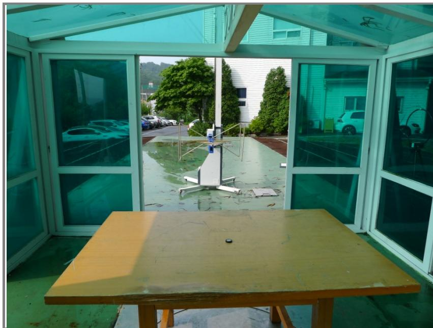
**Photo of radiated spurious emission at above 1 000 MHz**
