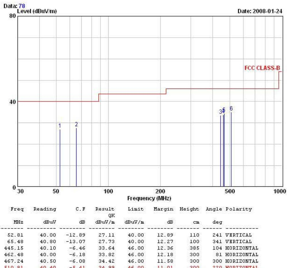
Remarks: C.F (Correction Factor) = Antenna factor + Cable loss - Preamp gain
