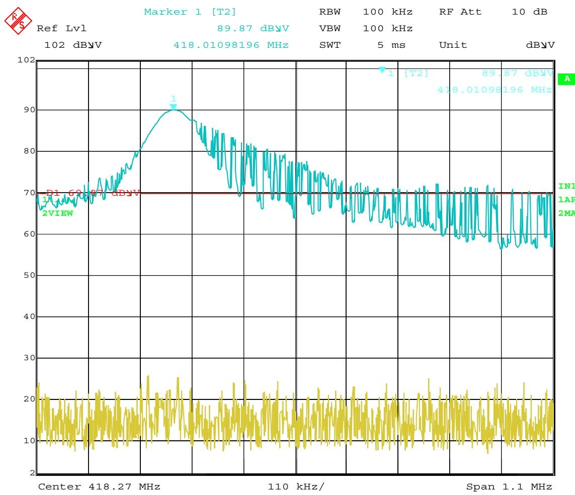
Reference Level of Fundamental Emissions for 20 dB Bandwidth
