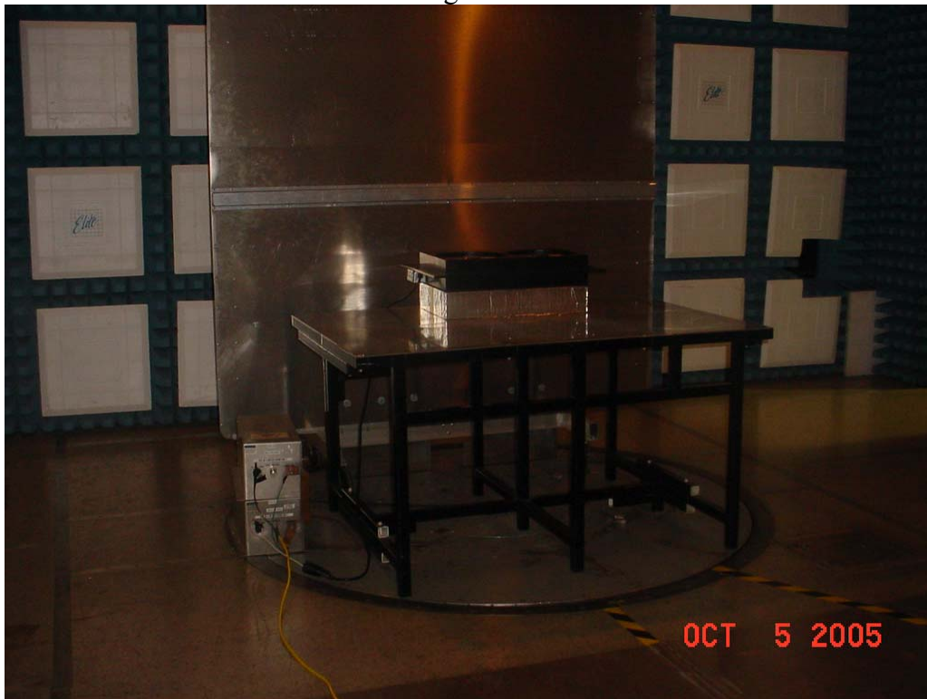
Test Setup for Conducted Emissions
