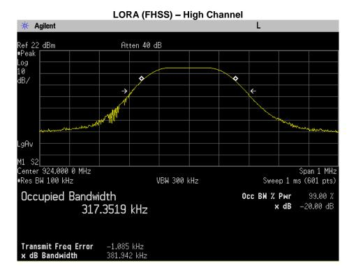
**Transmitter Power Spectral Density (PSD)**
