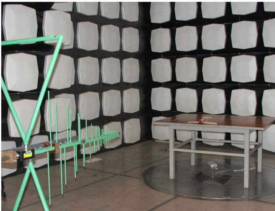
Radiated Emission Test Set-up (Receiver, Vertical)
