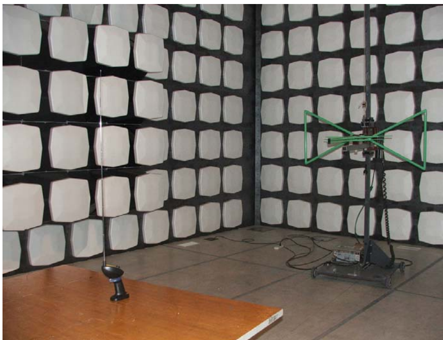
Field Strength within Band Test Set-up (Horizontal)
