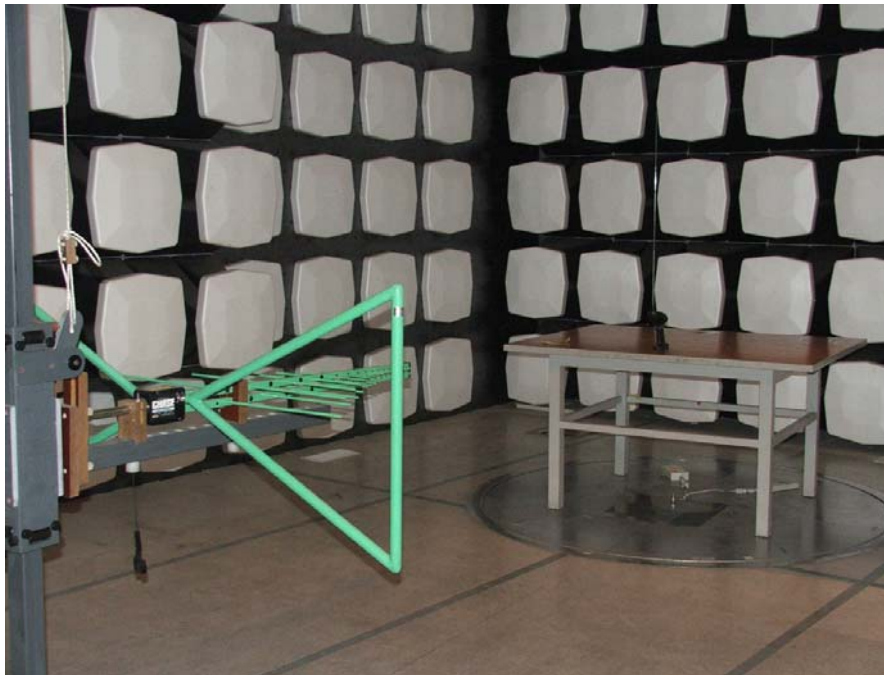
RADIATED EMISSION TEST Set-up (Transmitter, Horizontal)
