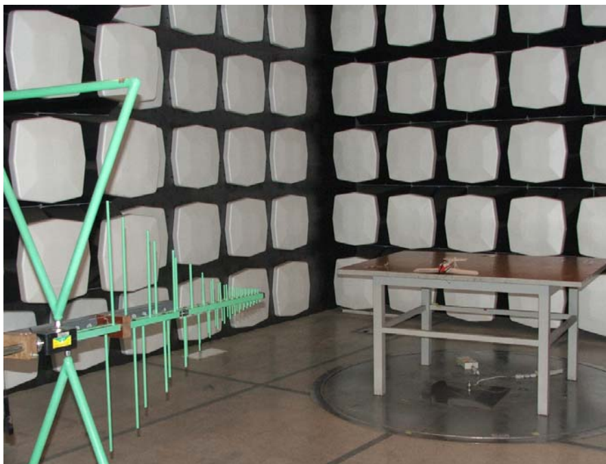
RADIATED EMISSION TEST Set-up (Receiver, Vertical)
