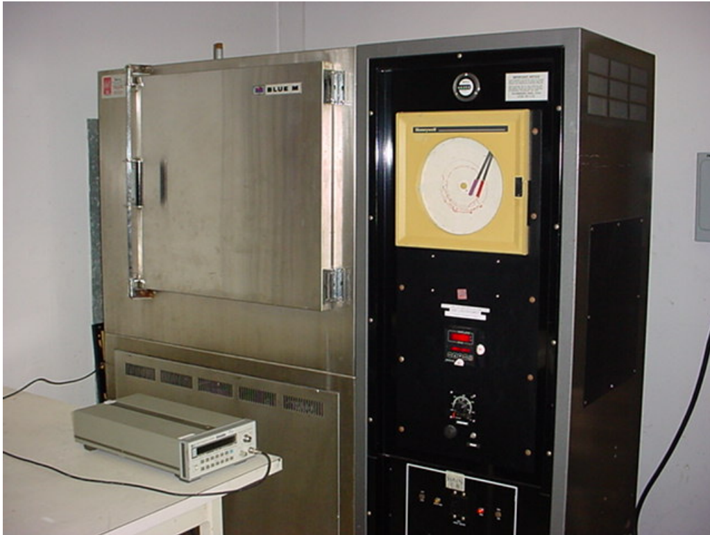
Frequency Tolerance Measurement Test Set-Up
