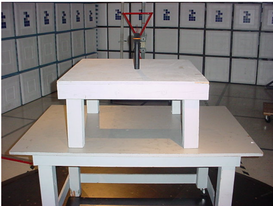
Transmitter Spurious EMI Measurement Test Set-up
