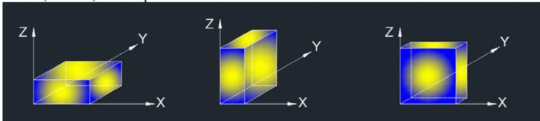
Note: For all radiated test, EUT in each of three orthogonal axis emissions had been tested, but only the worst case (Y axis) data recorded in the report.
