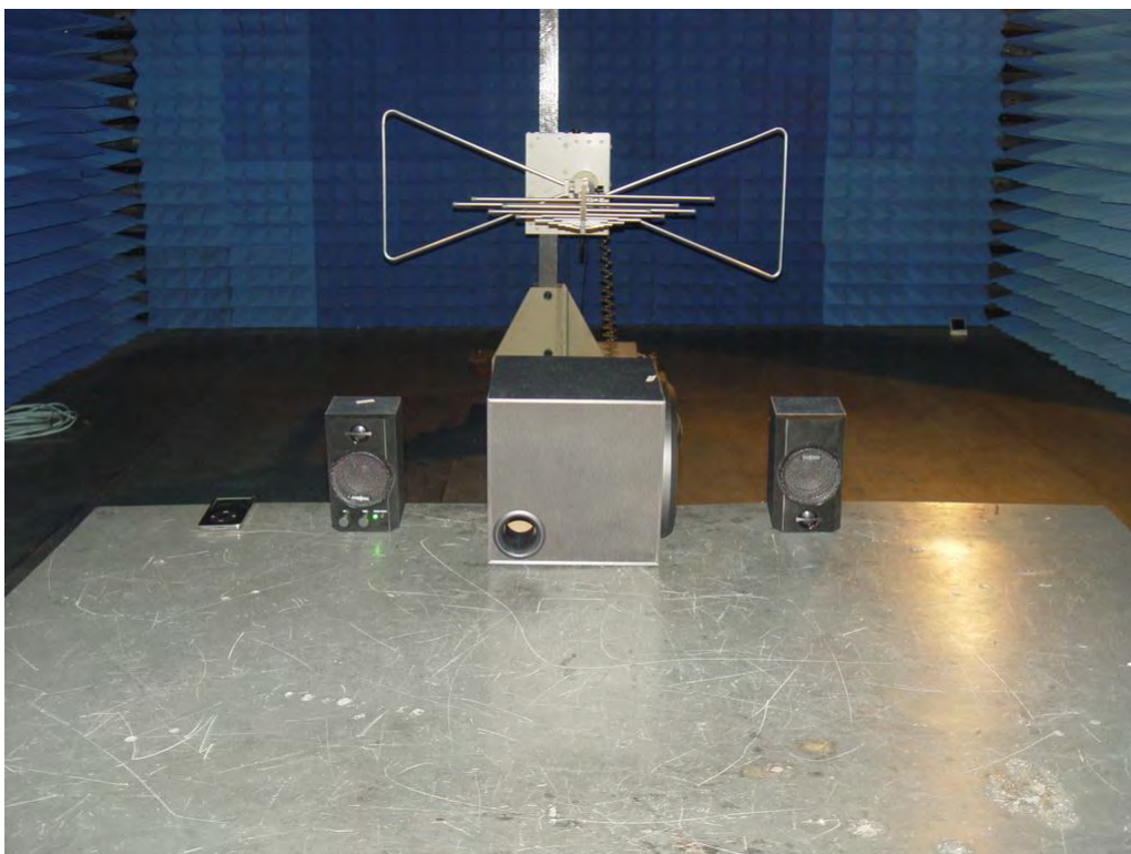
Photograph 2: Set-up for Radiated Emissions
