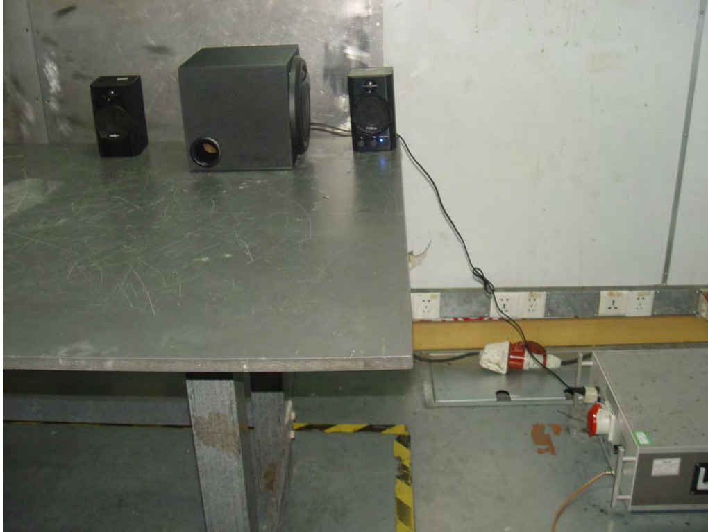
Photograph 2: Set-up for Radiated Emissions
