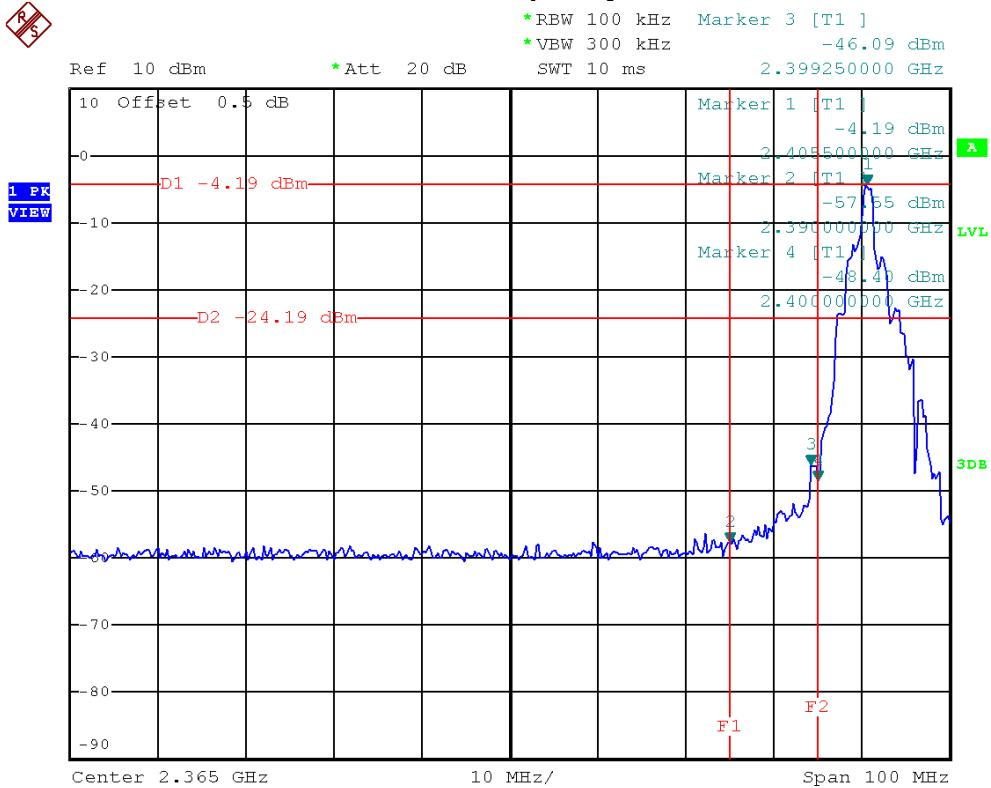
**The max. radio frequency power in any 100 kHz bandwidth within the frequency band**
