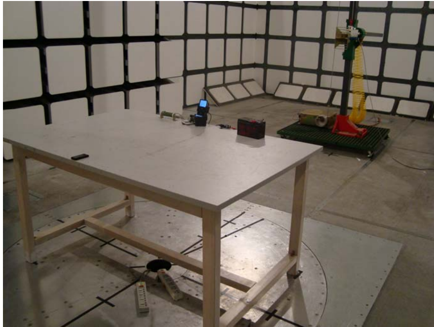
Radiated Emissions - Front View (above 1 GHz)
