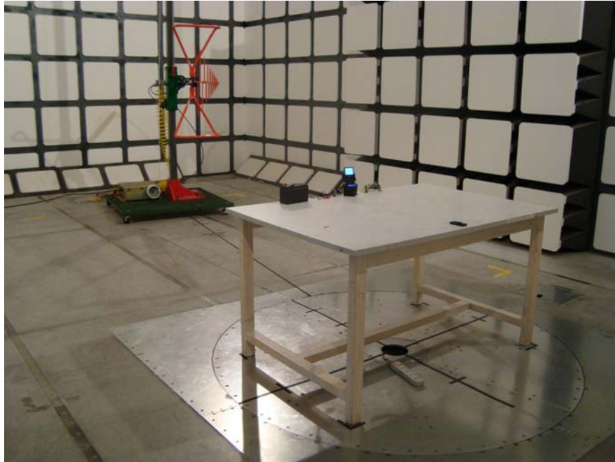
Radiated Emissions - Rear View (below 1 GHz)
