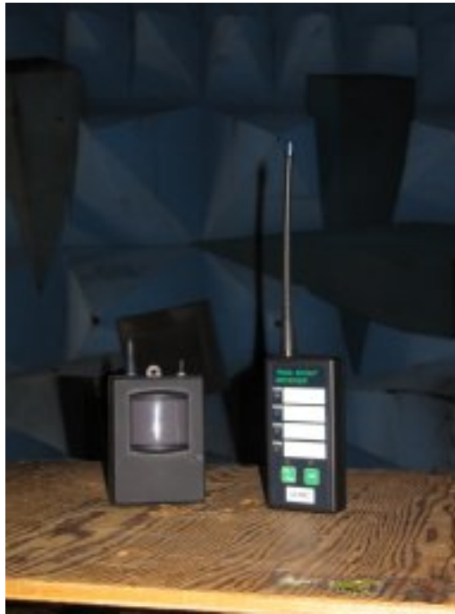
Figure 4.3a: Setup of sensor and receiver at 3-meters from antenna
