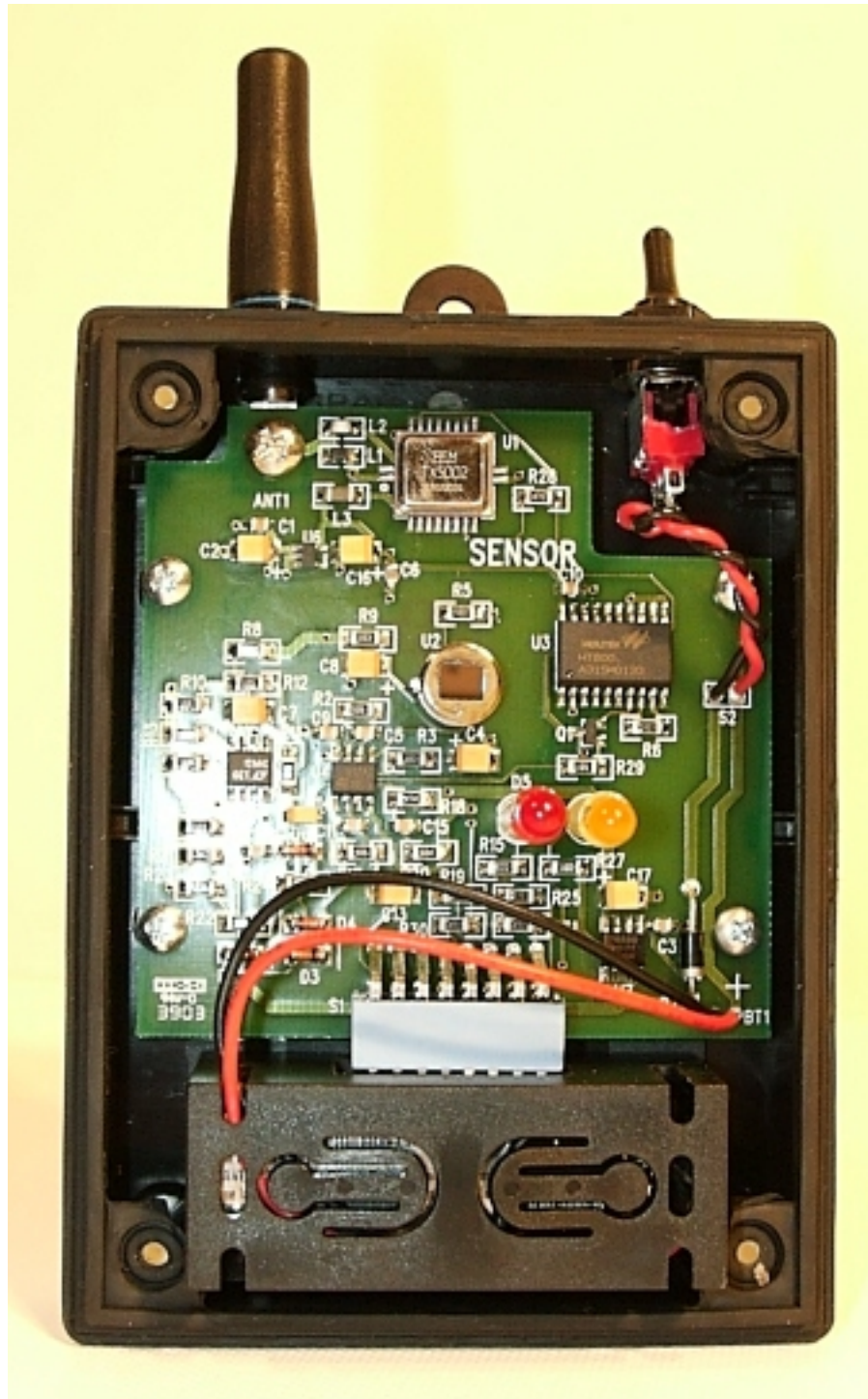
Photograph 6: Sensor Unit – Disassembled, Component Side
