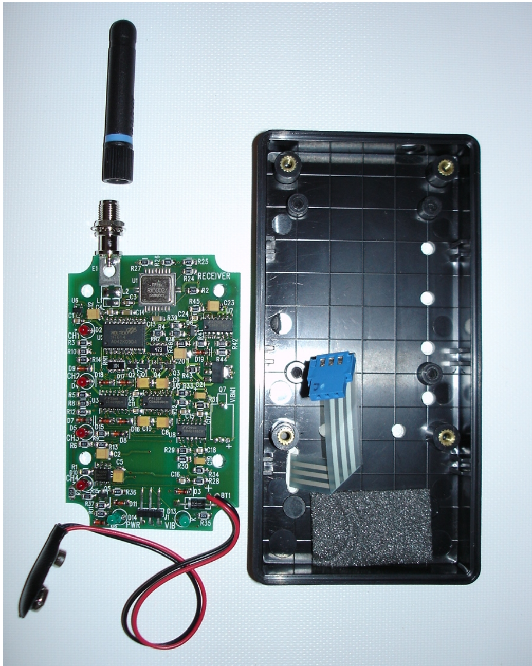
Photograph 4: Receiver Unit – Disassembled, Component Side
