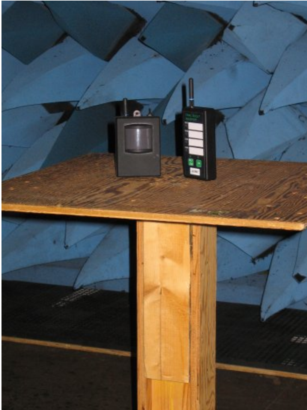
Photograph 1: Setup of Sensor and Receiver Unit (Short Antenna)
