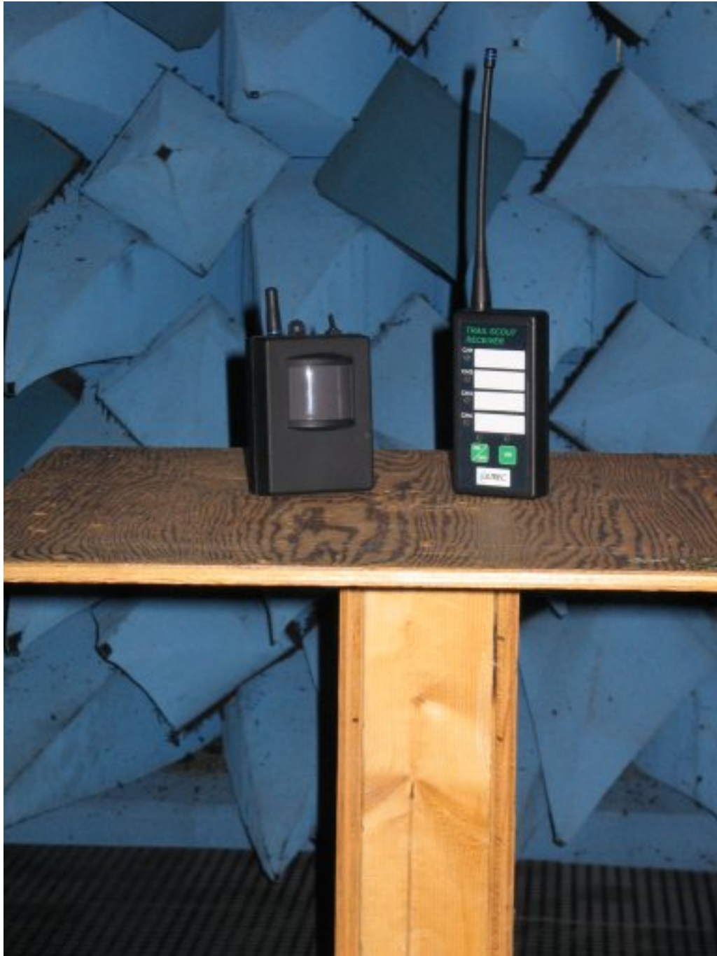
Photograph 2: Setup of Sensor and Receiver Unit (Long Antenna)
