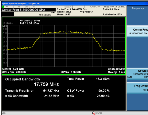
802.11ac_VHT20 UNII 2C BAND 26dB Bandwidth(CH 116)
