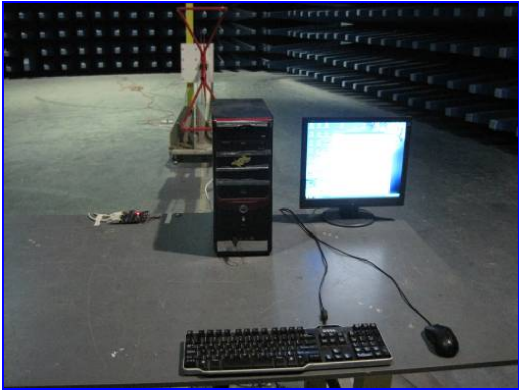
Front View of Radiated Emission Test Setup below 1GHz
