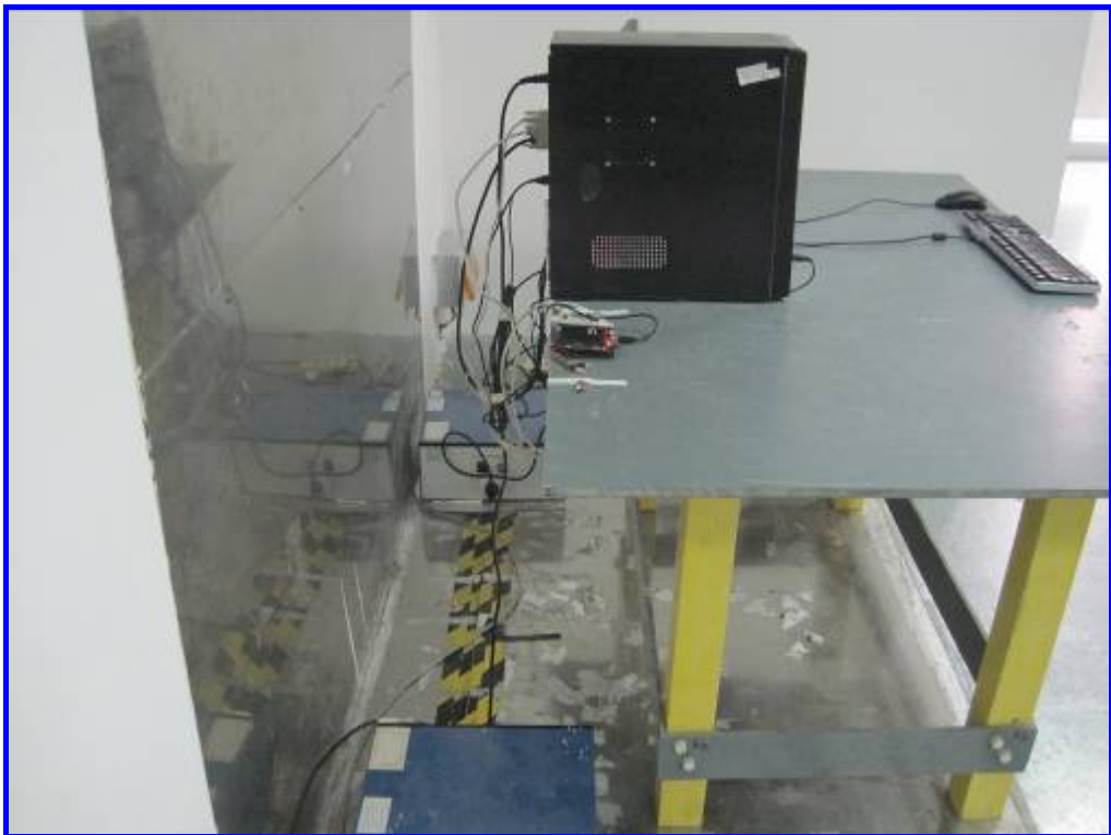
Side View of Conducted Emission Test Setup
