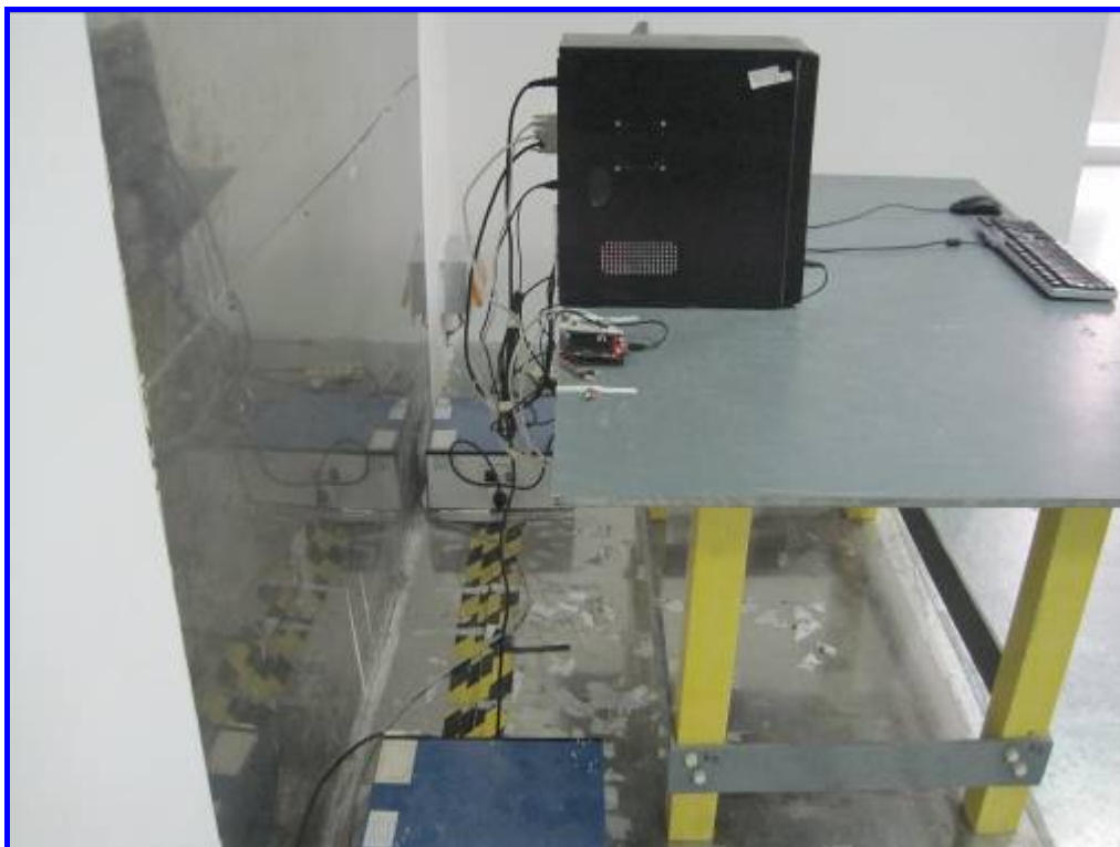
Side View of Conducted Emission Test Setup
