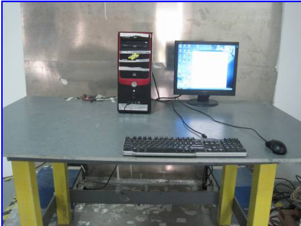
Front View of Conducted Emission Test Setup
