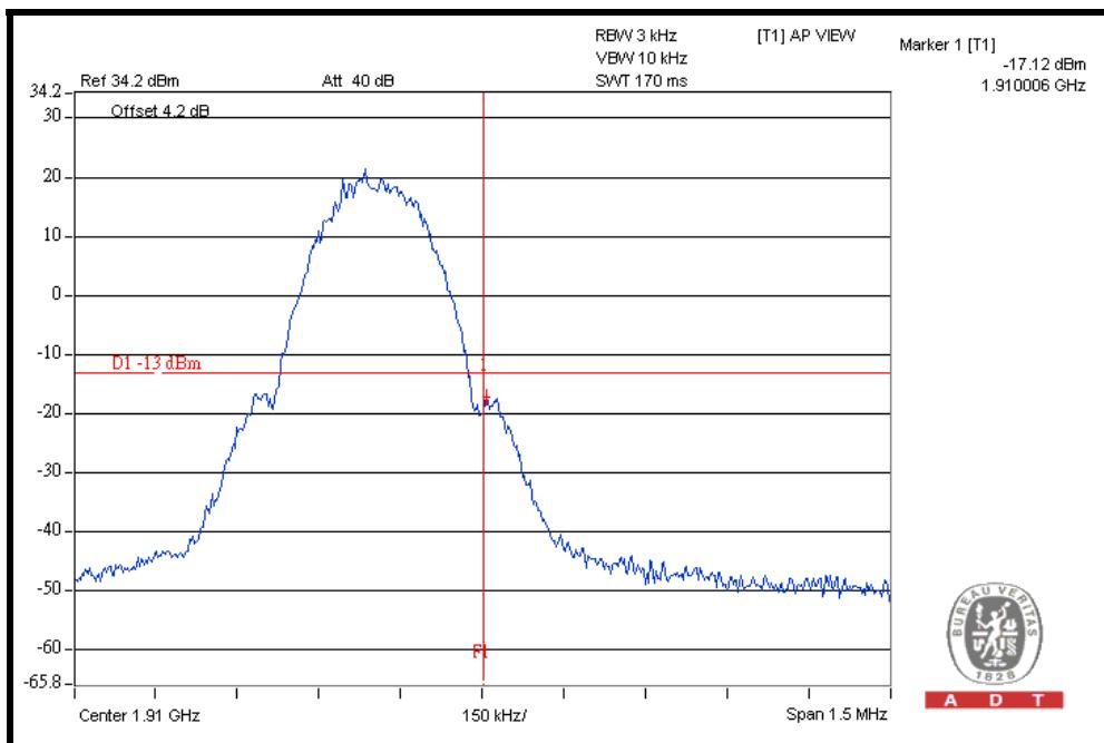
**FOR E-GPRS MODE (UP-LINK WITH 1 TIME SLOT)**
