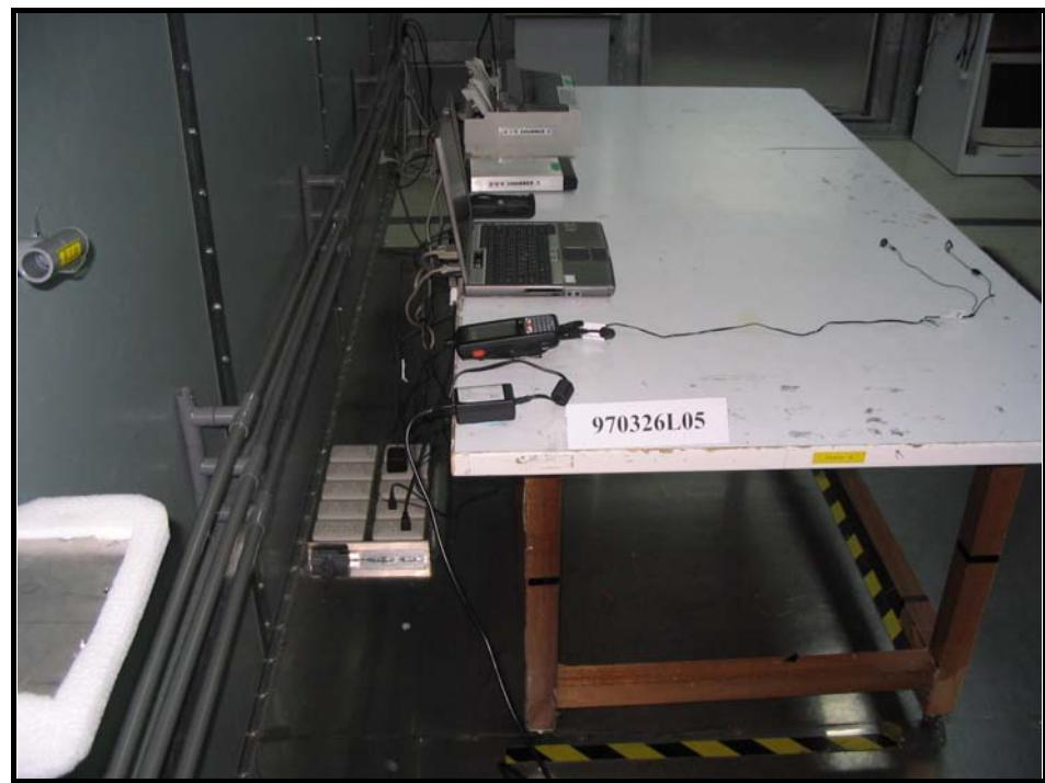
CONDUCTED EMISSION TEST (Test mode B2)
