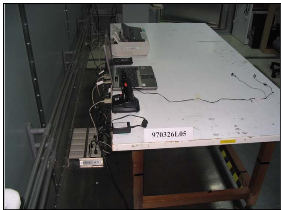
CONDUCTED EMISSION TEST (Test mode B1)
