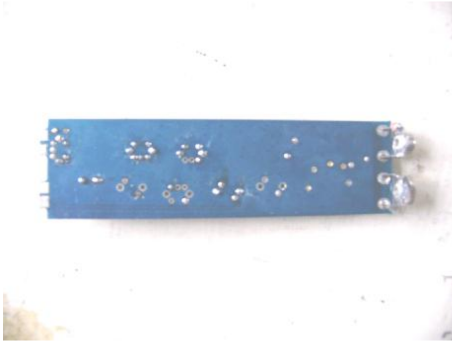
Tx Main board solder side
