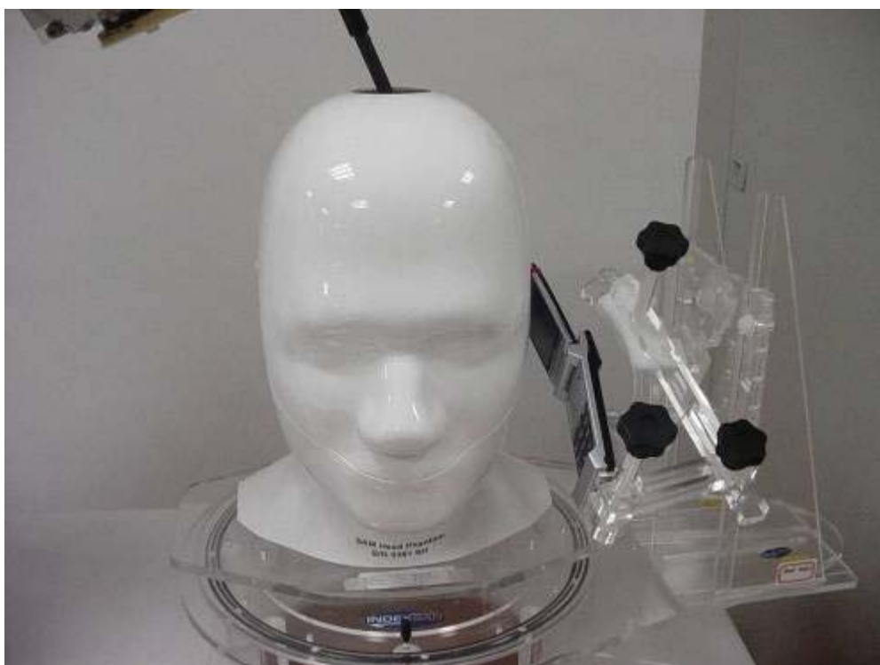
Fig.4 EUT Left Head Tilt15 Position
