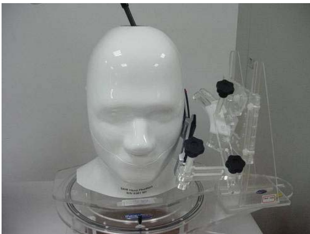
Fig.3 EUT Left Head Touch Cheek Position
