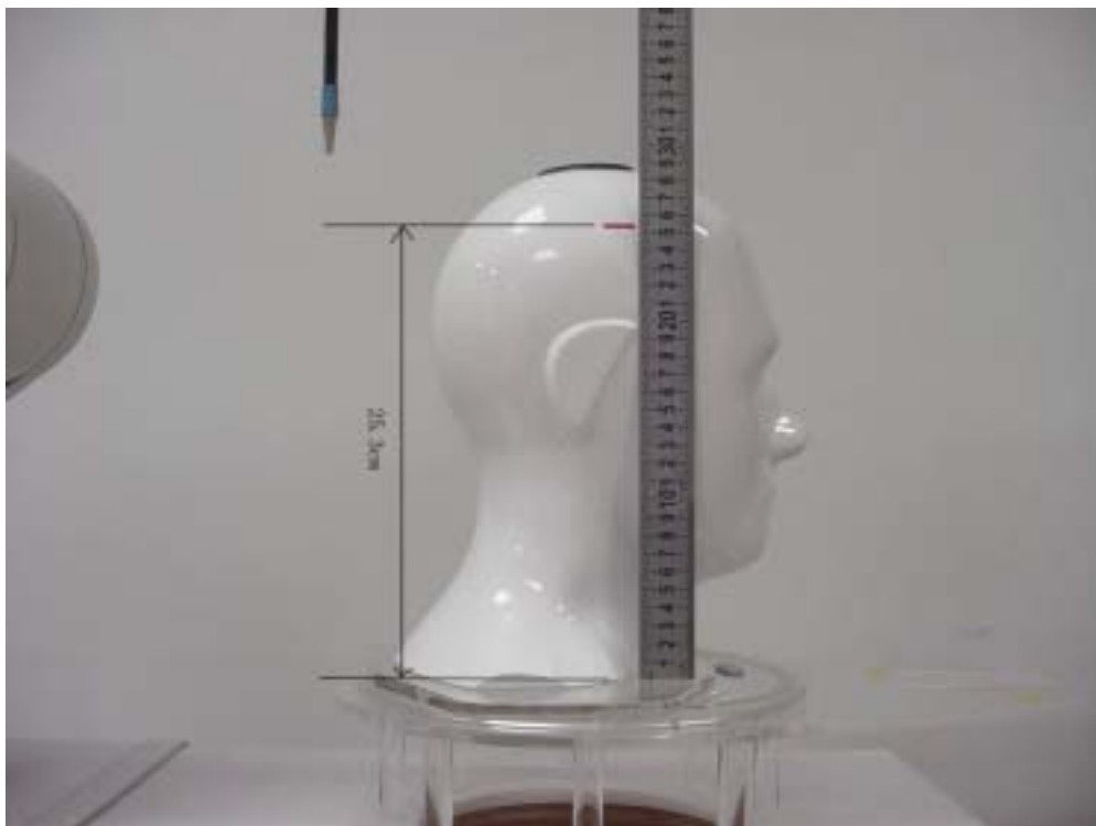
Fig.2 The depth of head tissue in SAM
