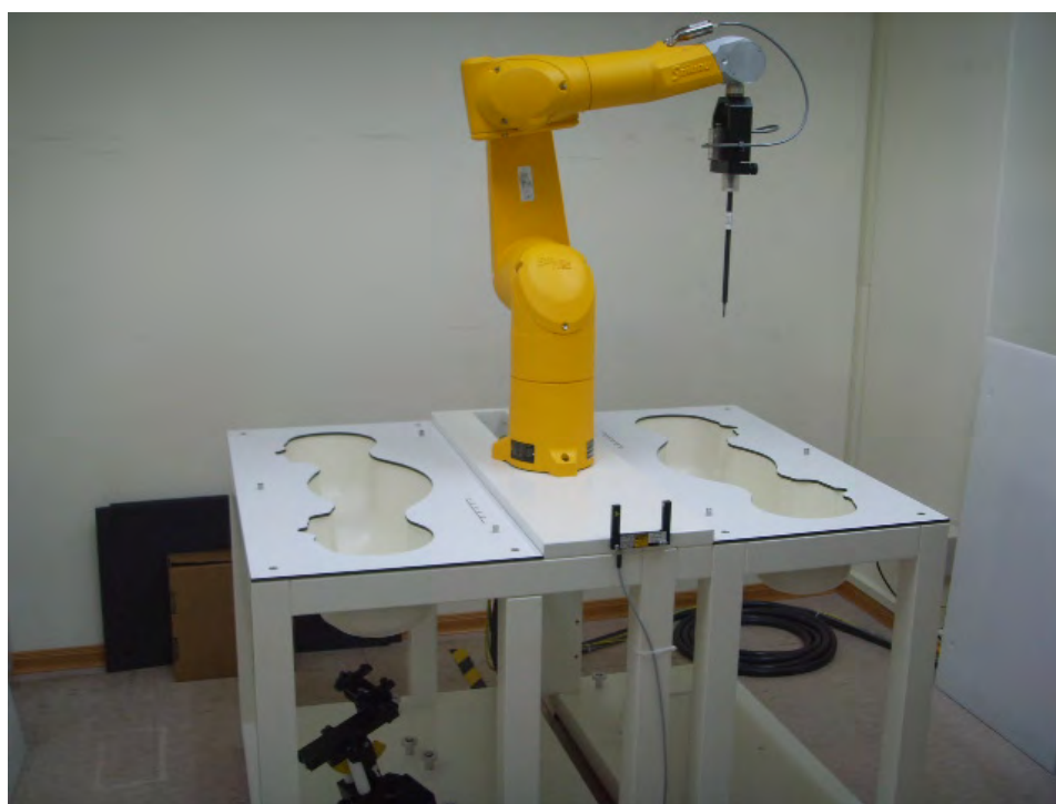
Fig.1 Photograph of the SAR measurement system
