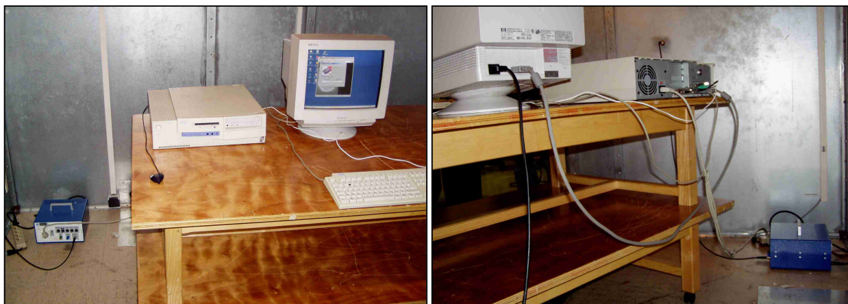
Conducted emissions test setup
