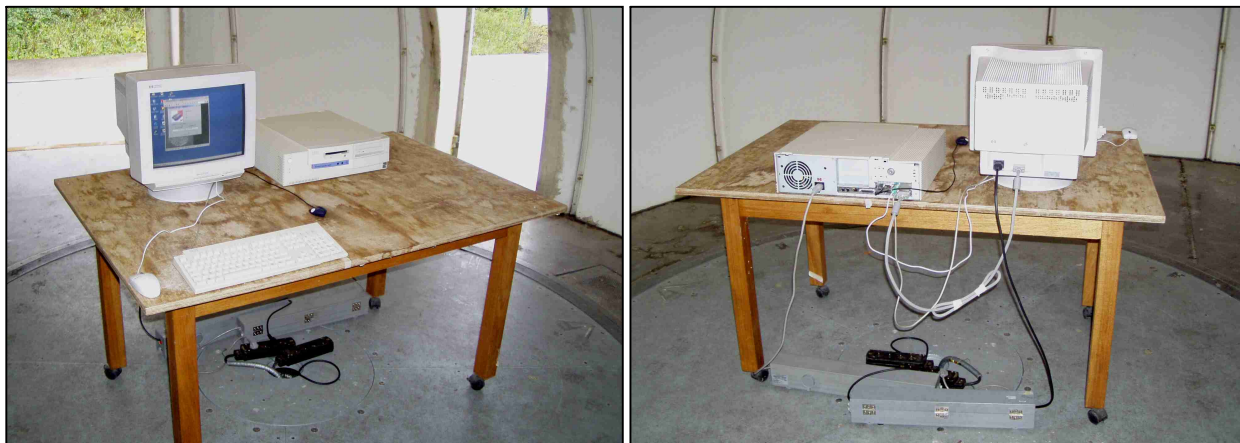
EUT 80cm above the ground reference plane
