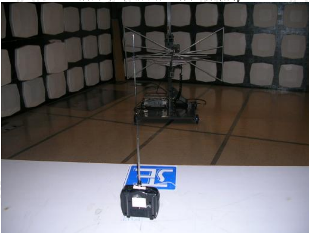
Measurement of Radiated Emission Test Set Up
