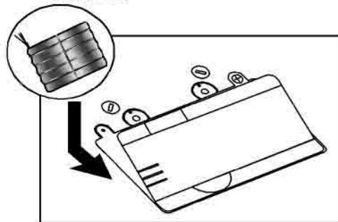
2. Slide supplied POWER CHARGE Battery into battery compartment and lock into place by turning compartment lock(as shown).
