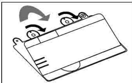
1. Open by turning the lock and lift the cover off.
