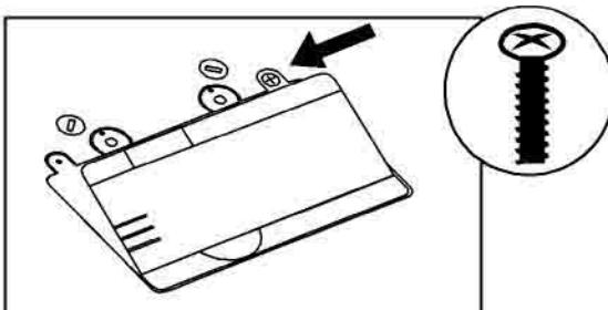
3. Place the cover to match the compartment, then slide cover down, and lock by tightening the screw.
