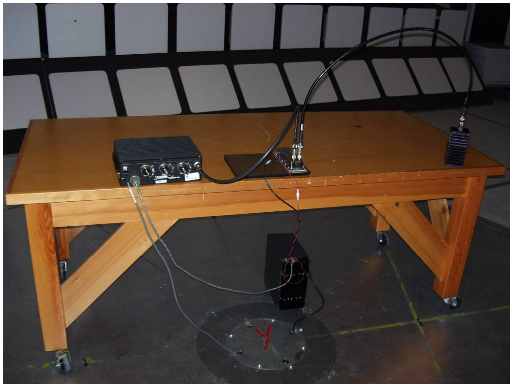
Figure 1 – Radiated Spurious Emissions Test Setup
