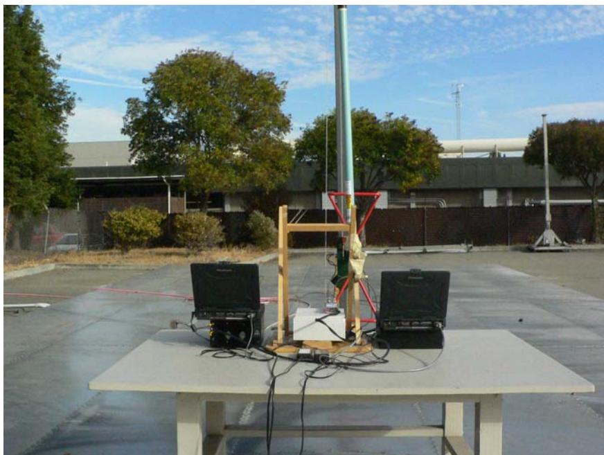
**Uplink Radiated Emission With AS Antenna - Front View**
