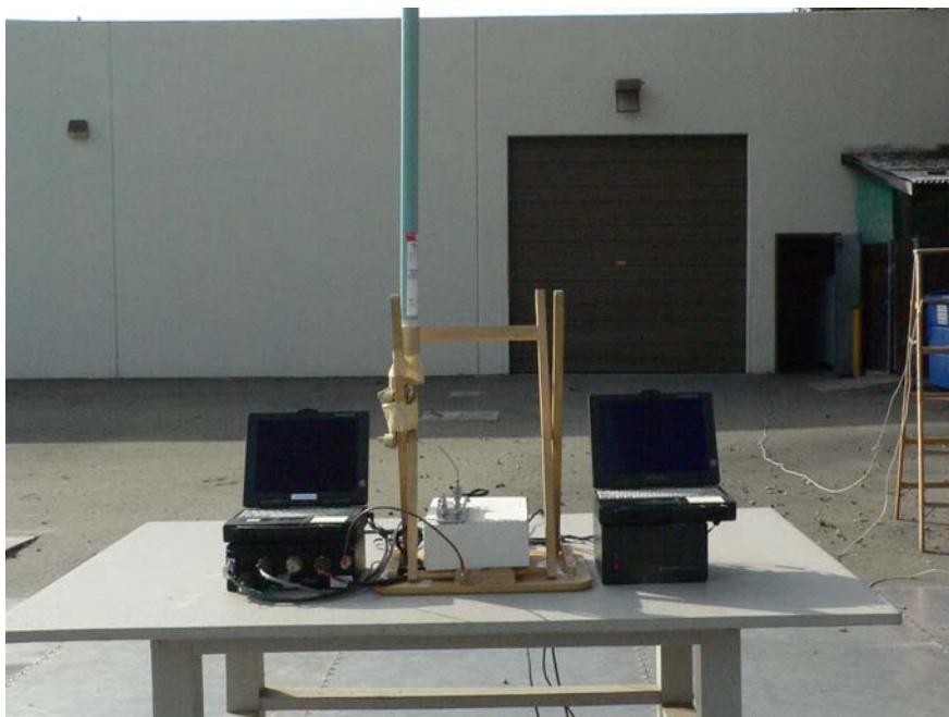
**Downlink Radiated Emission With Andrew Vertical Antenna - Rear View**
