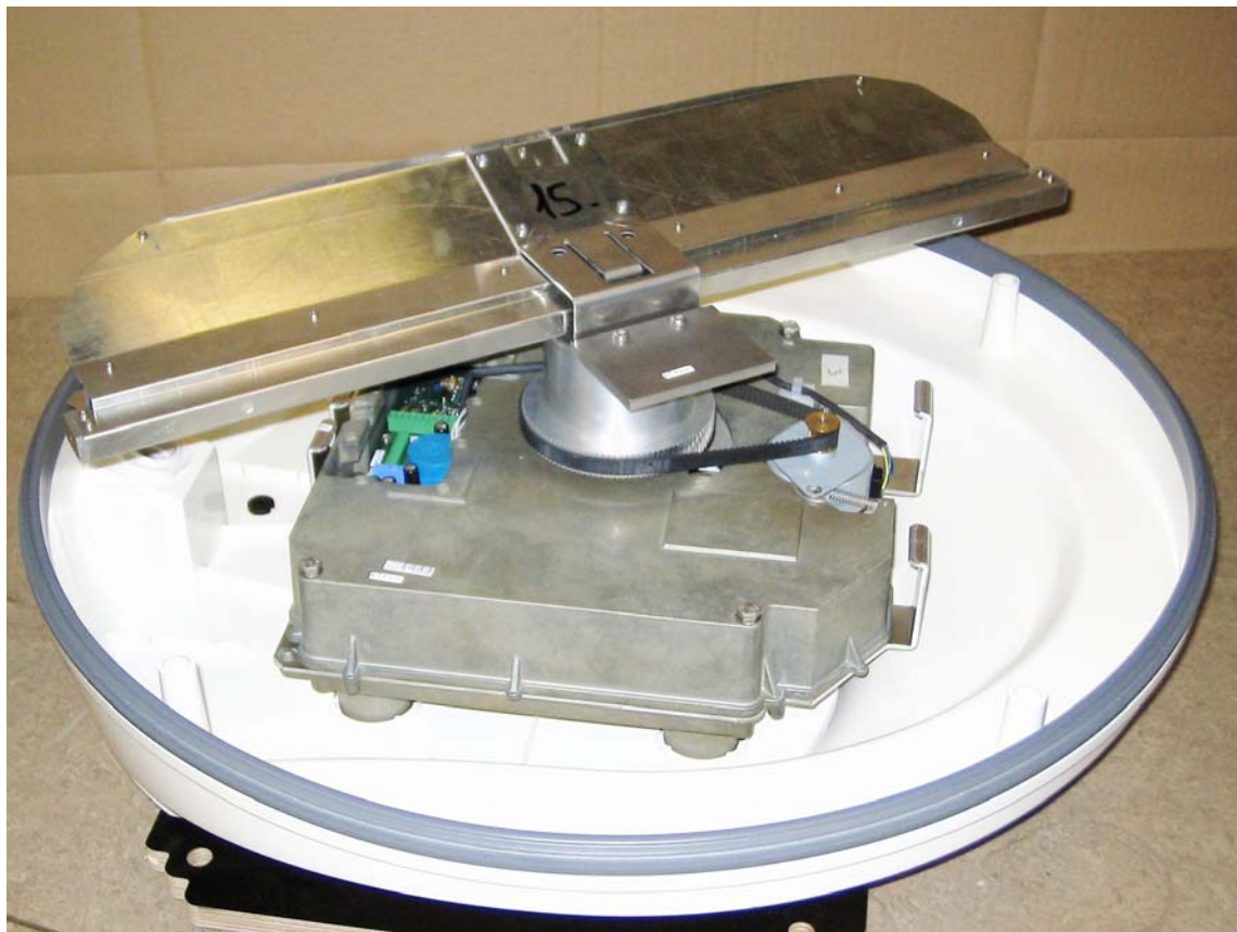
Figure 3 DX 45/60 absorber removed
