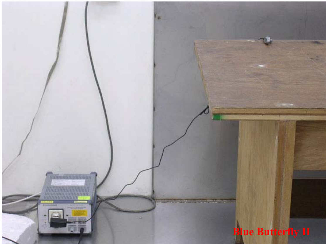
Photo 1: Conducted Emission Test Set-up photo
