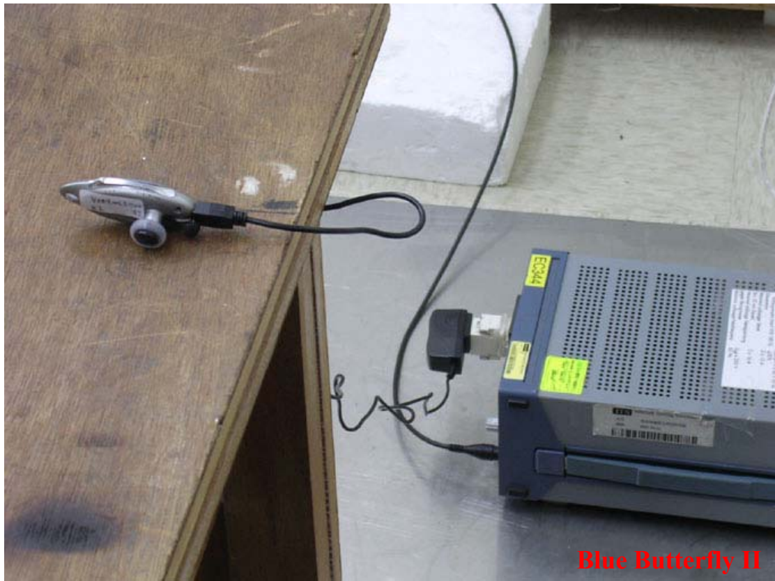
Photo 2: Conducted Emission Test Set-up photo
