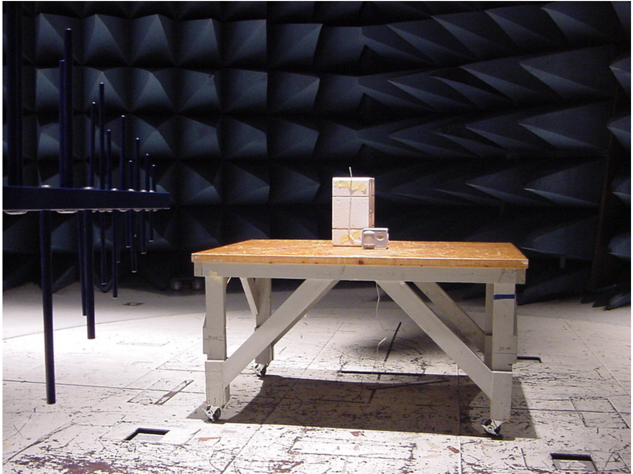
Photograph 4: Radiated Emission Test Setup < 1 GHz
