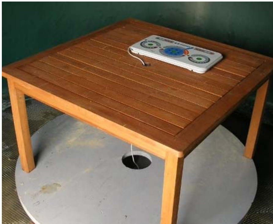
Radiated emissions test set up
