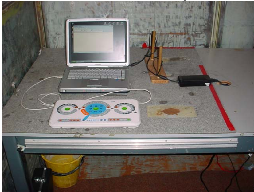
Conducted emissions test set up
