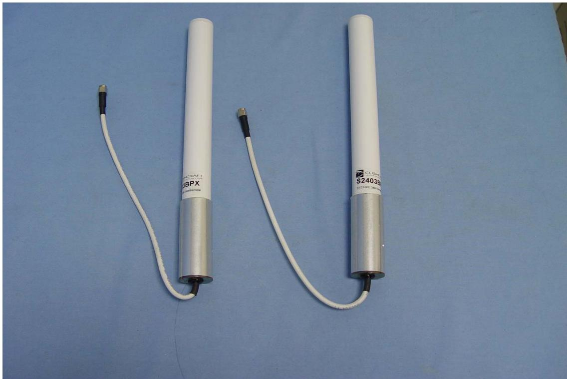
**Omnidirectional Panel antenna for 2.4G and 5G / 3.0 dBi**
