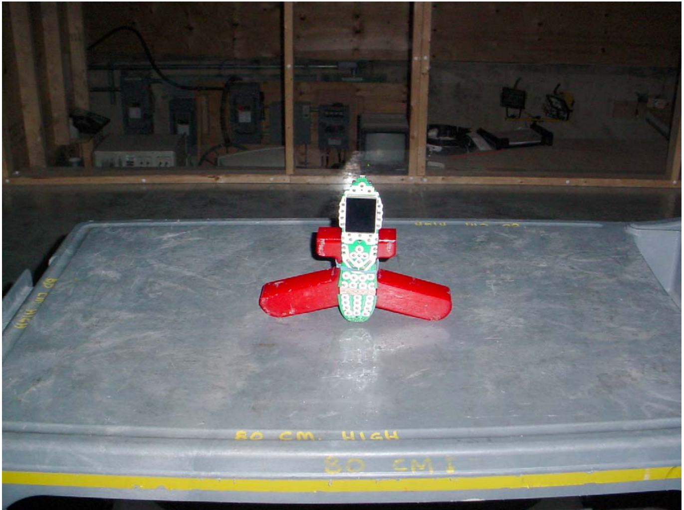
Radiated Emissions at 3 Meters EUT with Rigid Wire Antenna
