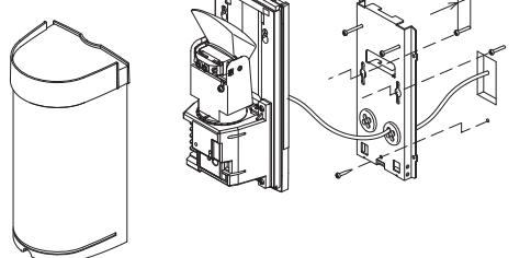
\* The grommet is compatible with a wire of  $\phi 0.12"$  ( $\phi 3mm$ ) to  $\phi 0.24"$  ( $\phi 6mm$ ) outer diameter.
