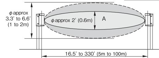
A core detection area is approximately  $\phi 2'$  (0.6m) as indicated above as A, when the alignment is correctly adjusted. It is suggested to make at least 3.3' (1m) open space on either side of detection area to prevent false alarm.
