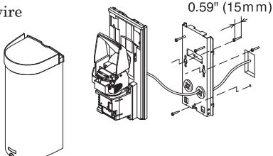
\* The grommet is compatible with a wire of  $\phi 0.12"$  ( $\phi 3mm$ ) to  $\phi 0.24"$  ( $\phi 6mm$ ) outer diameter.
