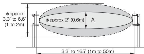
A core detection area is approximately  $\phi 2'$  (0.6m) as indicated above as A, when the alignment is correctly adjusted. It is suggested to make at least 3.3' (1m) open space on either side of detection area to prevent false alarm.
