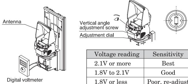
After adjustment, set the adjustment mode switch to "Operation mode".
