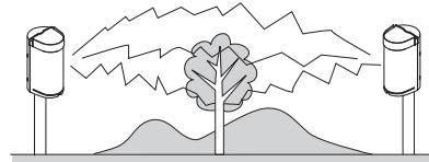
Note: Install the sensor at a proper height and position otherwise detection area could be widened over 6.6' (2m).
