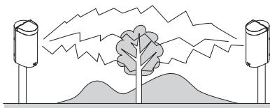
Note: Install the sensor at a proper height and position otherwise detection area could be widened over 6.6' (2m).
