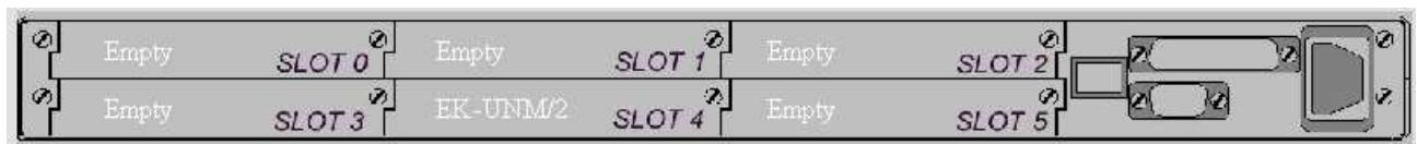
The EK-UNM/2 board is loaded in the slot number four; to visualize the web page of the board is necessary to move, using a mouse, the cursor on the slot associated to the board (slot 4) and then to click the left mouse button on its. So we obtain the following image:
