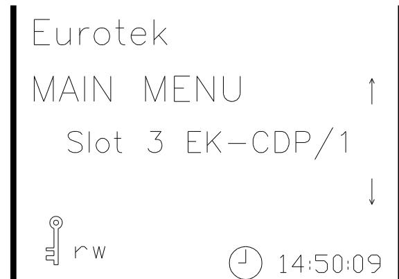
Pressing the “enter” key, (*EK-MFR/1 user ‘s handbook, front panel description* paragraph) the user can enter to the EK-CDP/1 menu and using the “explore menu” keys it is possible to see the four main menu of the board: Status, ODU RX Set, ODU TX Set and Revision.
