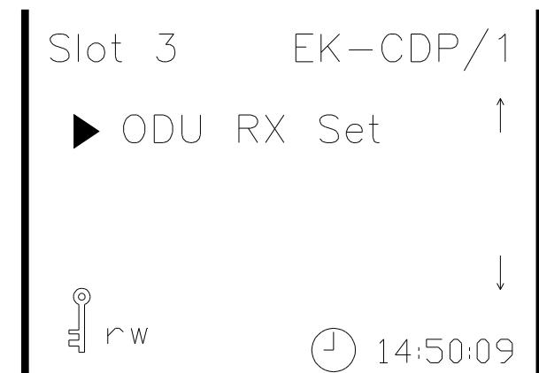
When the ODU RX Set menu is selected (above view), pressing the “enter” key it is possible to enter in the sub-menu of the ODU RX Set menu and, using the “explore menu” keys, to run until the Rx menu as follow:
