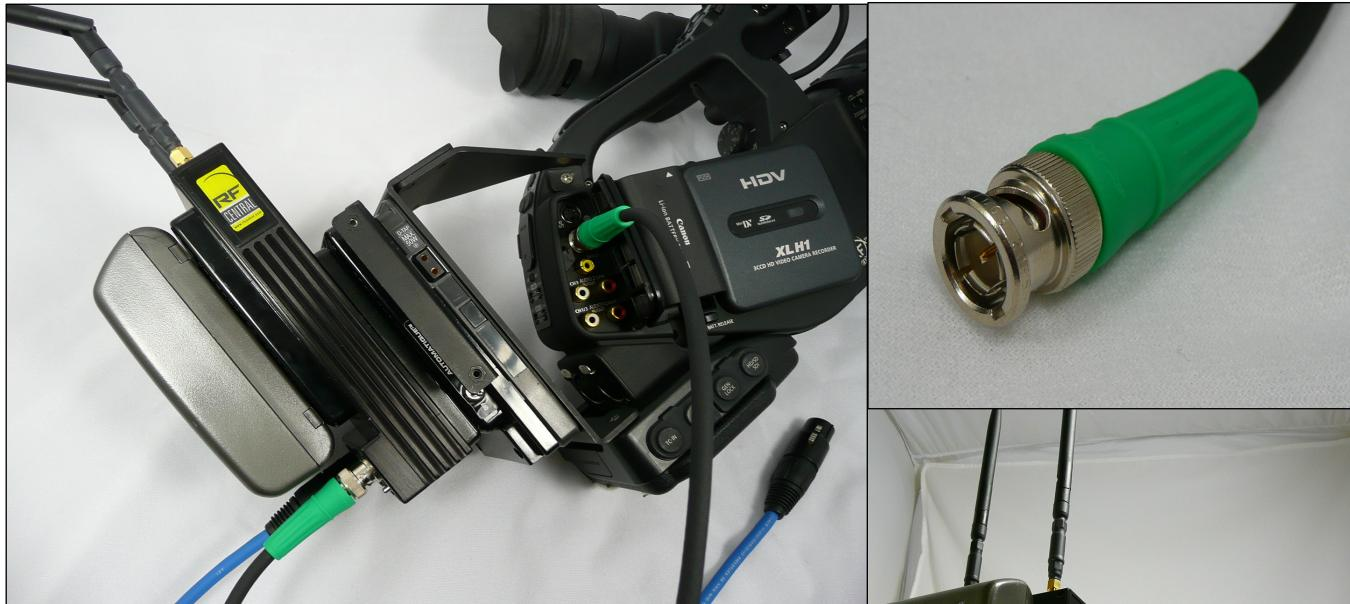
Plug one end of the Video cable into the BNC connector on the camera, and the other end into the BNC connector on the transmitter.
