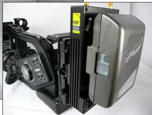
Clip camera battery on back of transmitter.
