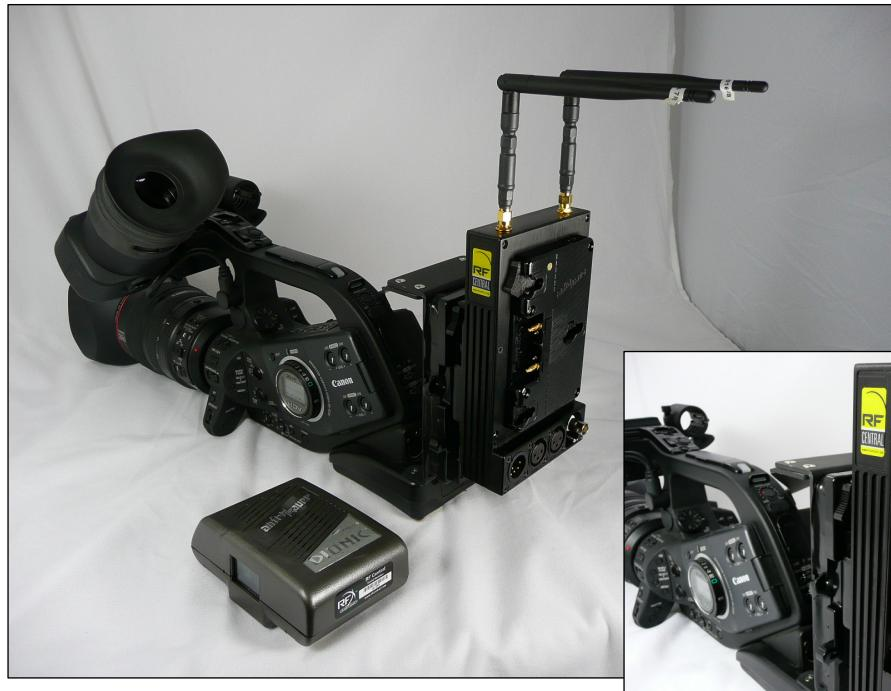
Place the transmitter on the back of the camera.
