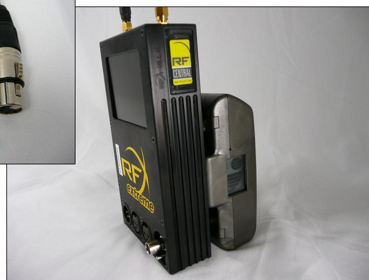
Supply the receiver with 8-18v DC from a battery or power supply via the 4 pin XLR.
