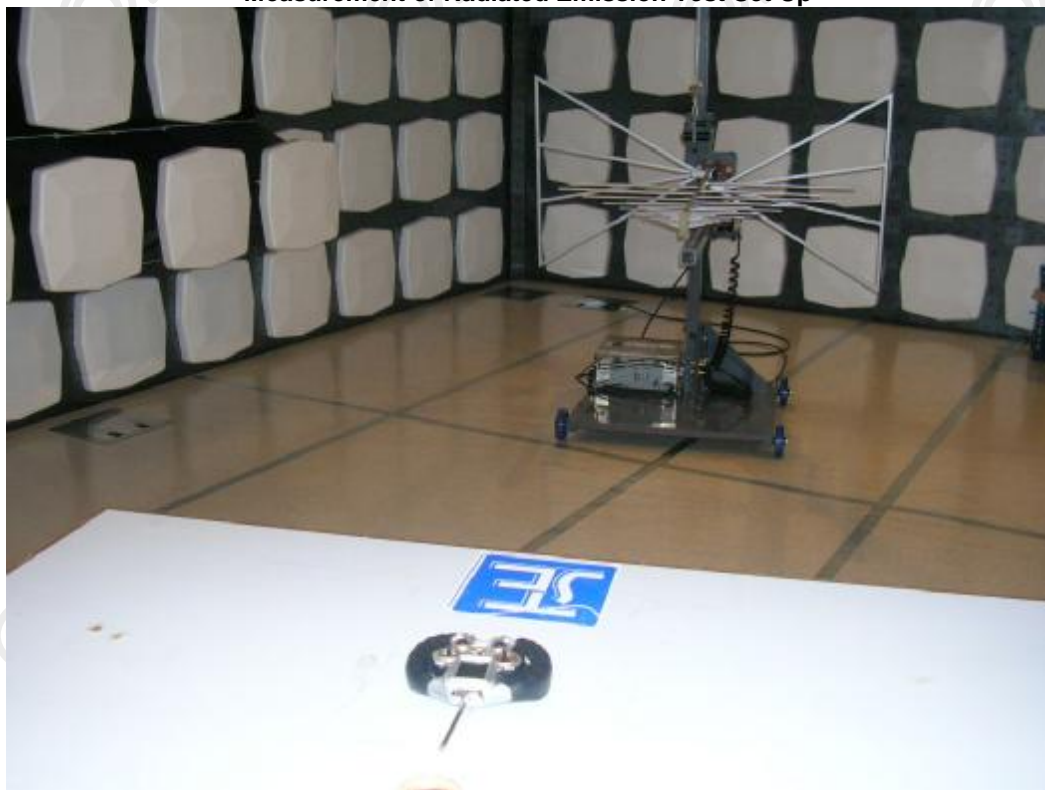
Measurement of Radiated Emission Test Set Up
