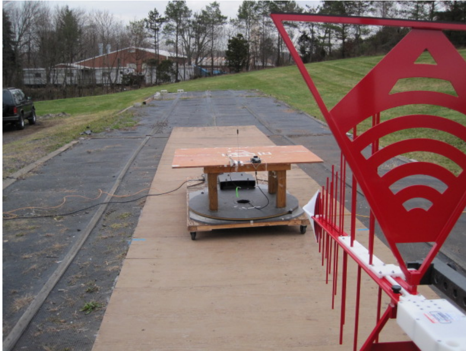
Vertical Antenna Polarization
