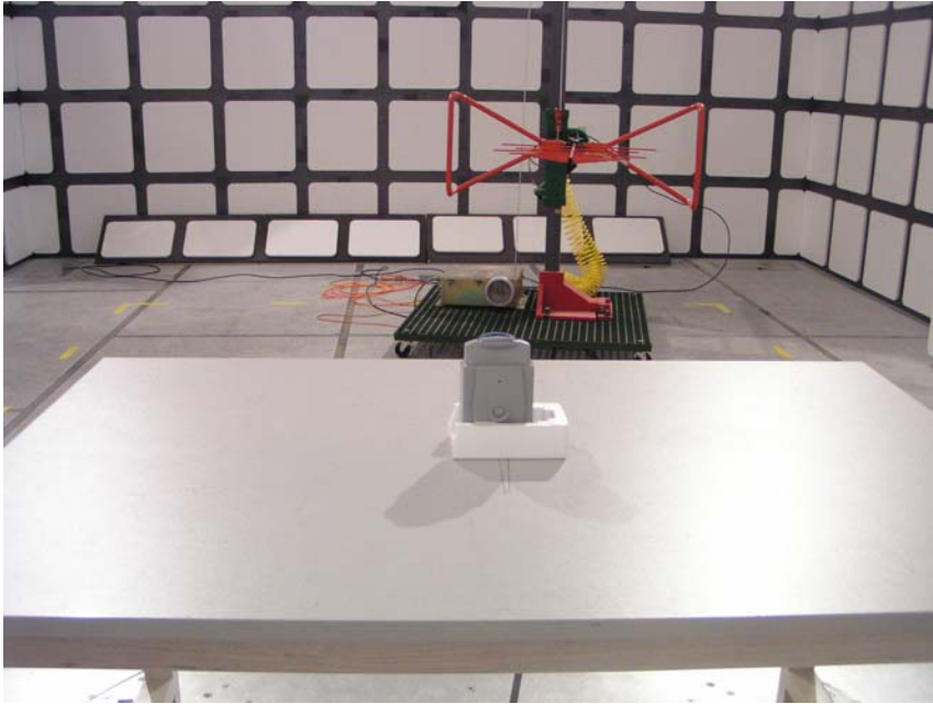
Radiated Emissions-Front View
