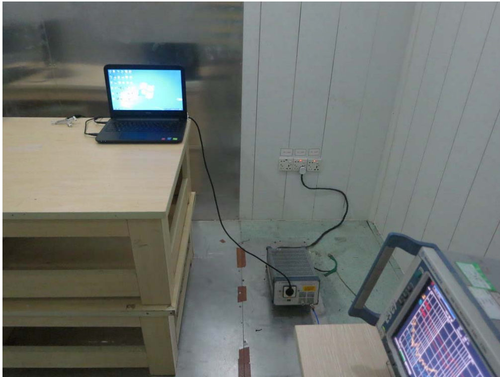
FCC RADIATED EMISSION TEST SETUP
