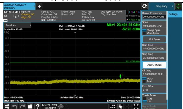
802.11n(HT40),2422MHz,Ant0,Plot 2,Band Edge
