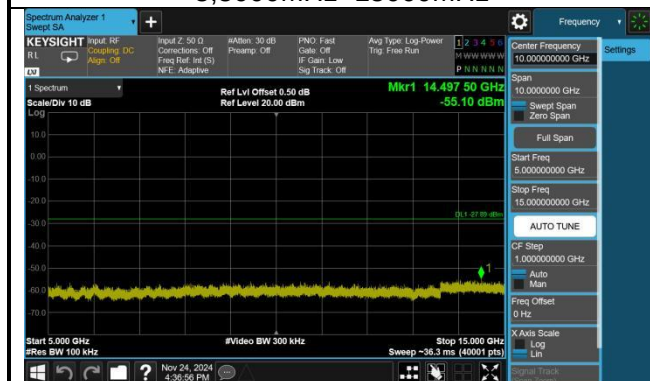
802.11n(HT40),2422MHz,Ant0,Plot 1,Reference Level
