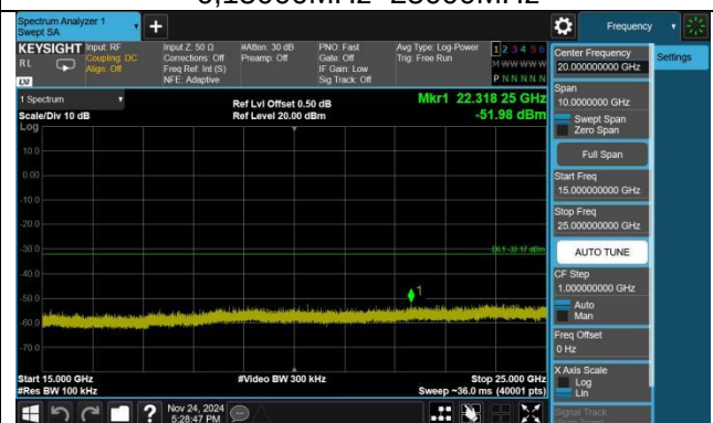
802.11n(HT40),2437MHz,Ant0,Plot 2,Band Edge
