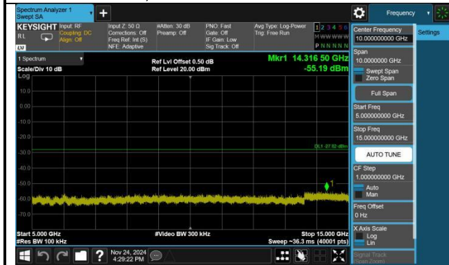
802.11n(HT20),2462MHz,Ant0,Plot 1,Reference Level
