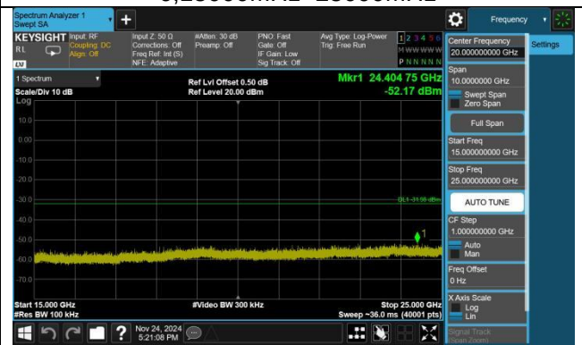
802.11n(HT40),2452MHz,Ant0,Plot 2,Band Edge
