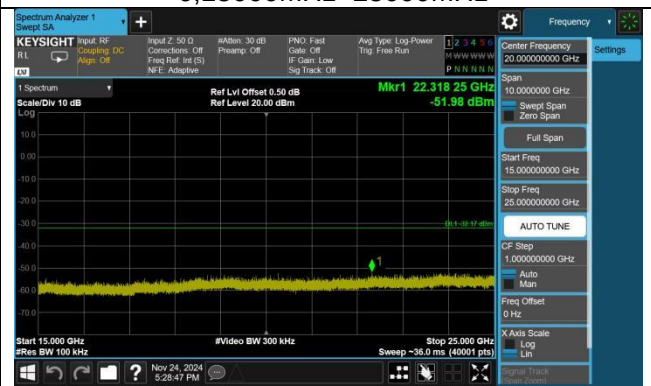
802.11n(HT40),2437MHz,Ant0,Plot 2,Band Edge
