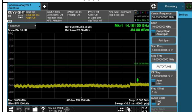
802.11n(HT20),2412MHz,Ant0,Plot 1,Reference Level
