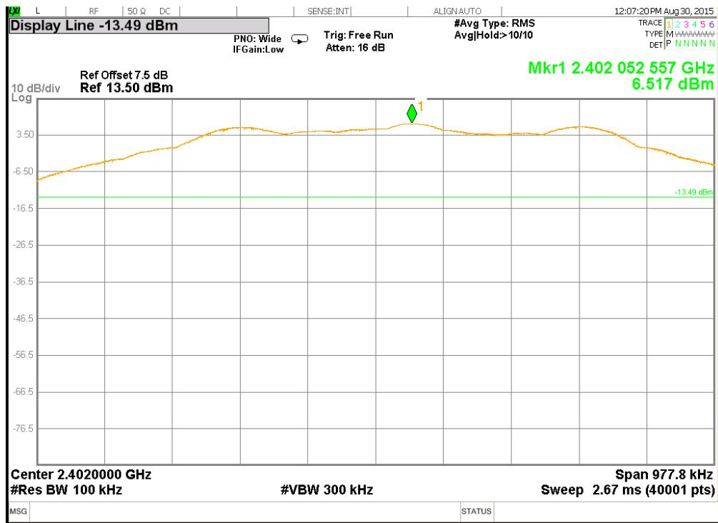
Chain0 : Conducted Spurious @ GFSK mode Low Channel
