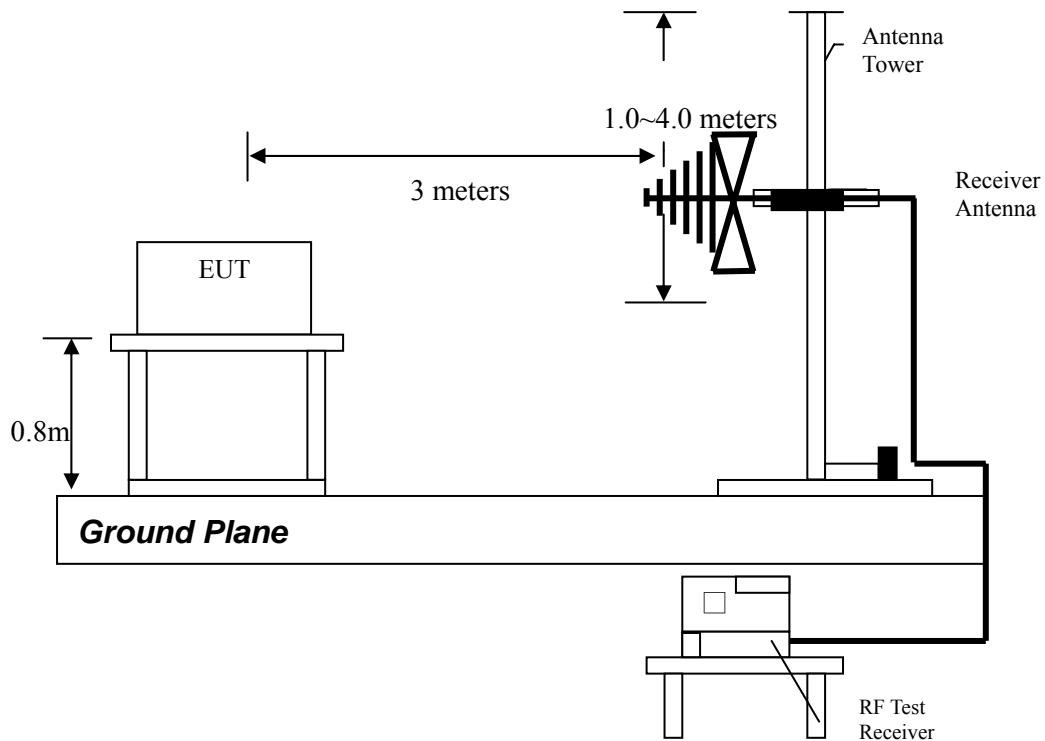
**7.5.3 Radiated emission above 1GHz using Horn Antenna**
